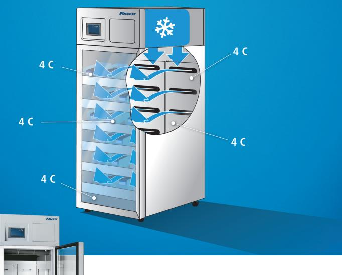
Ever see shelves loaded heavily or unevenly? Blocked airflow in other manufacturers' refrigerators and freezers could leave areas out-of-temperature.
