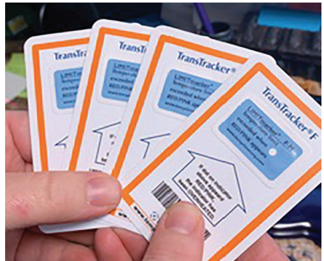
TransTracker F monitors medication for heat excursions and provides a visual indication for the patient on receipt
